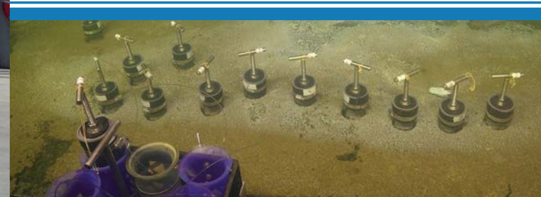
Above: Pushcores inserted by ROV Jason into a microbial mat for analysis of geochemical parameters and microbial community composition.
